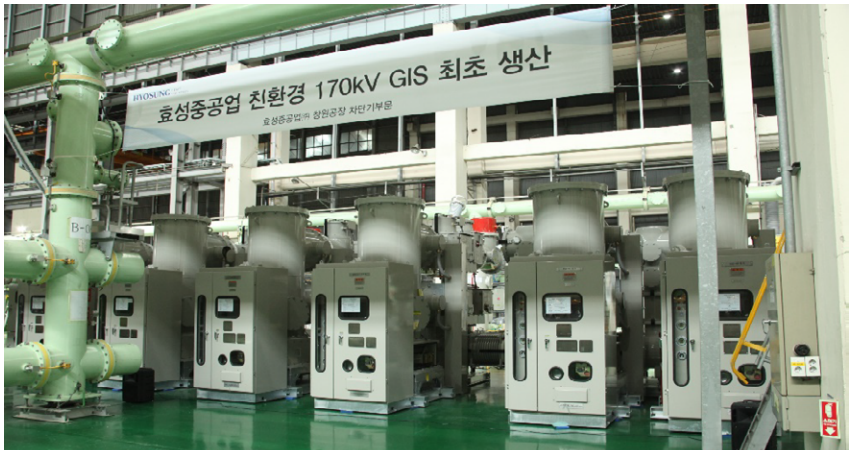
170kV 50kA GIS with Novec mixture gas
