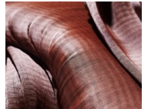
Tire cord made from recycled PET yarn
