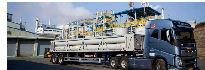
Tube trailer high-pressure hydrogen tank
